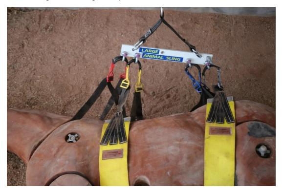
Once all the 2" webbing has been attached, adjust the straps to shorten the distance from the spreader bar to the back of the animal. Because the 4" webs are positioned at the center of the animal, the adjustment of these webs should be equal, that is both adjustment lengths of the "yellow" connectors should be the same.
