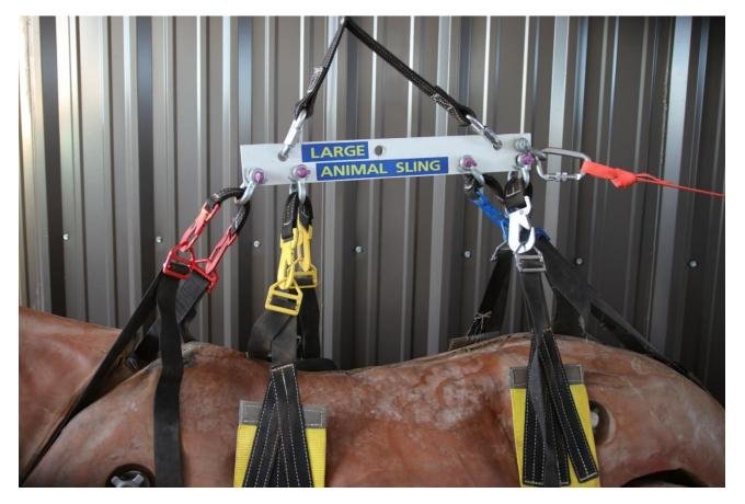
Attach an "anchor" strap or web to the rear of the spreader bar to help prevent the animal from "launching" forward in the lift when the horse becomes upright.
